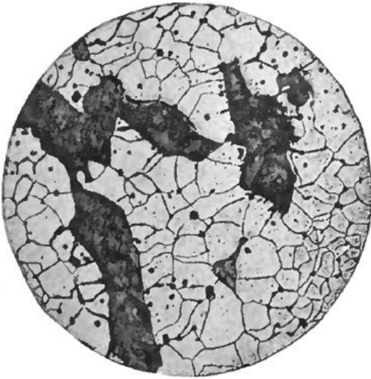
Fig. 4. — Wrought iron. Transverse section. Magnification not stated. (Guillet.)
